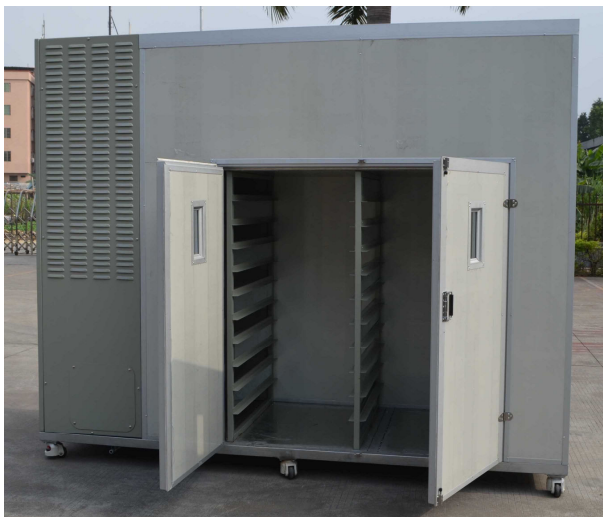
Rear view with space for 40 drying racks with 2 racks per level on 2 sides
