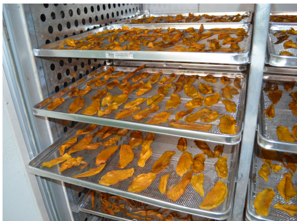
Rear view with space for 40 drying racks with 2 racks per level on 2 sides
